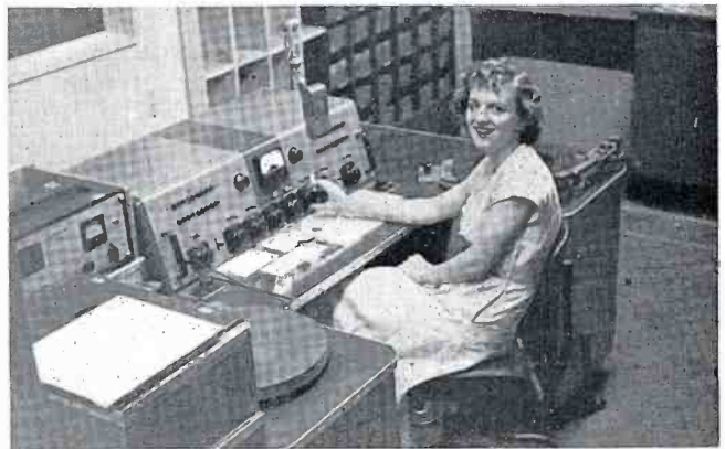
FIG. 5. A view of the control room of Radio Station WNAG. The RCA console and varicoustic mike are shown. The console operator faces a window separating the control room and the transmitter of WNAG. At WNAG the engineers also serve as announcers in a "Combination" type operation.
