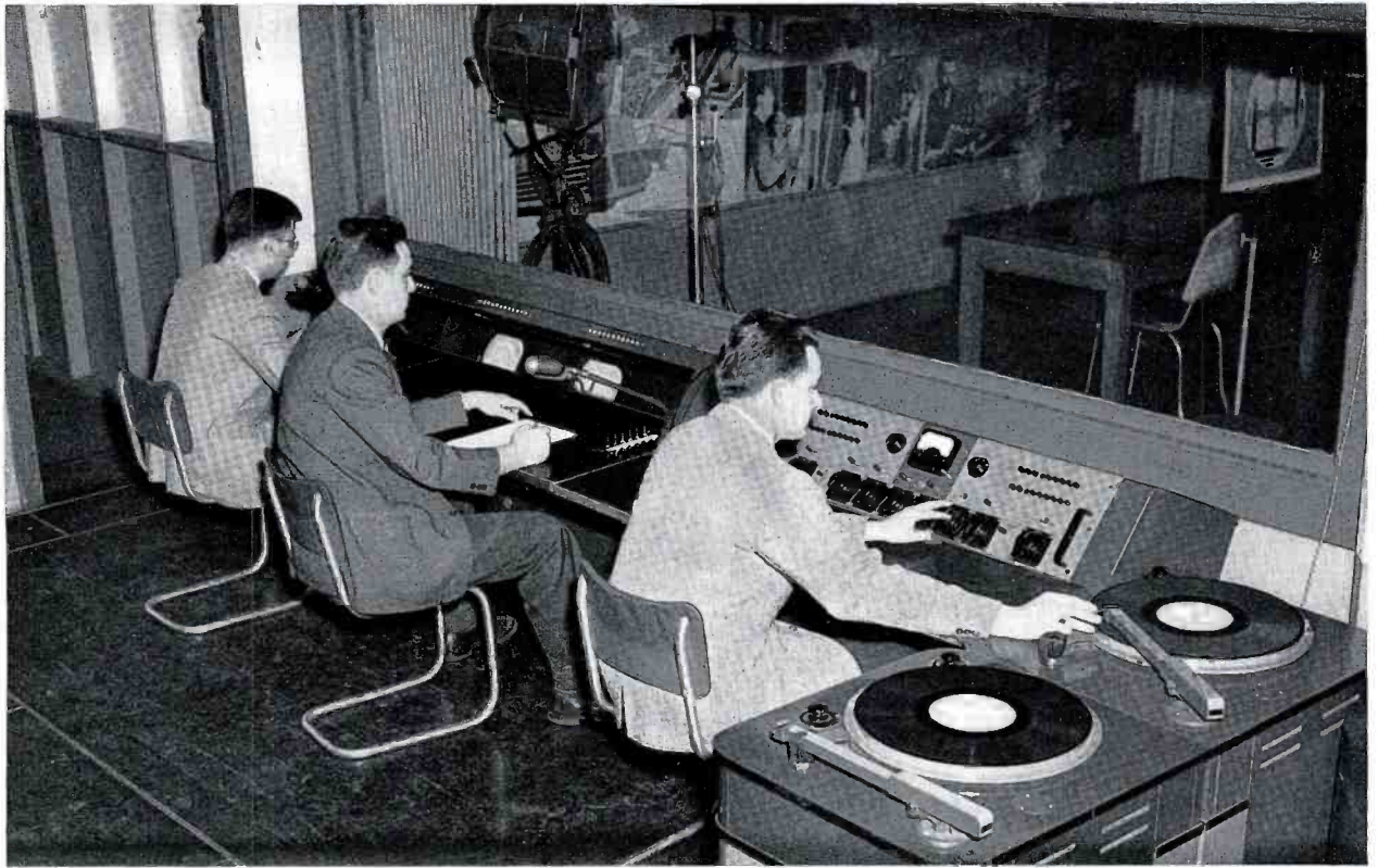
FIG. 6. Program Director's Console at left with Audio Console and Turntables in foreground.
