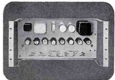
RCA GENLOCK, Type TG-45. This is the simple, automatic system that electrically locks two separate television pick-up systems together.
