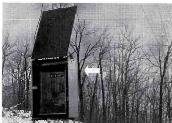
This special RCA Community Television Antenaplex Amplifier greatly intensifies the signals picked up on top of Sharps Mountain—assuring excellent reception in Pottsville homes.
