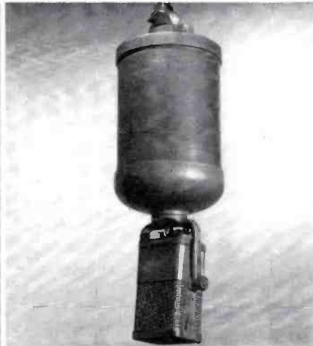
1930 An early model Ribbon Microphone (Velocity type). Note attached pre-amplifier and use of electromagnetic field.
