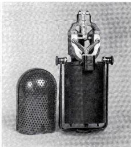
1936 The Type 77-A Universal (Ribbon) Microphone, forerunner of the present-day "77-D".
