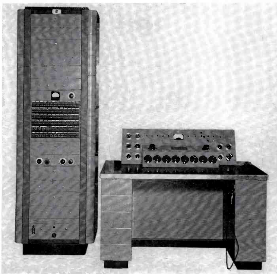
1948 Modern Broadcast Studio Control Console and companion audio equipment rack of the BR-84 series. Note matched appearance and styling of rack and console.
