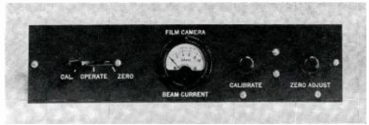
FIG. 13. Beam Current Metering Control Panel.
