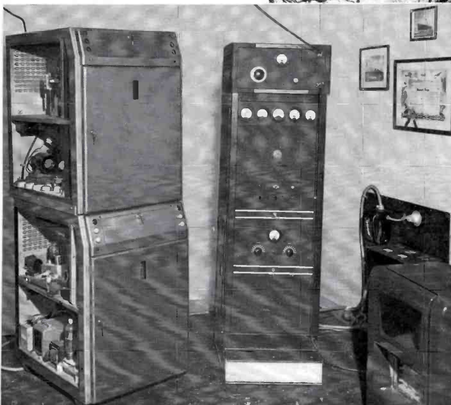
His present 500-watt transmitter (center) will be augmented with the new bandswitching KW under construction at the left.
