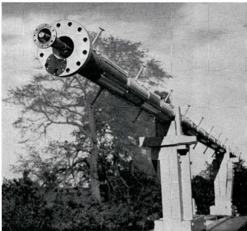
FIG. 3. Bottom View of TFU-24-BH Antenna Mounted on Turntable for Vertical Pattern Measurements. Showing Mounting Flange and Transmission Line Connection.
