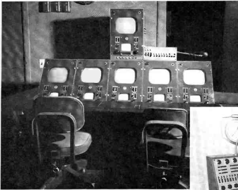
FIG. 4. Front view of video control console at El Capitan. Five monitors in console are associated with four live and one film cameras. Unit mounted above is master monitor.
