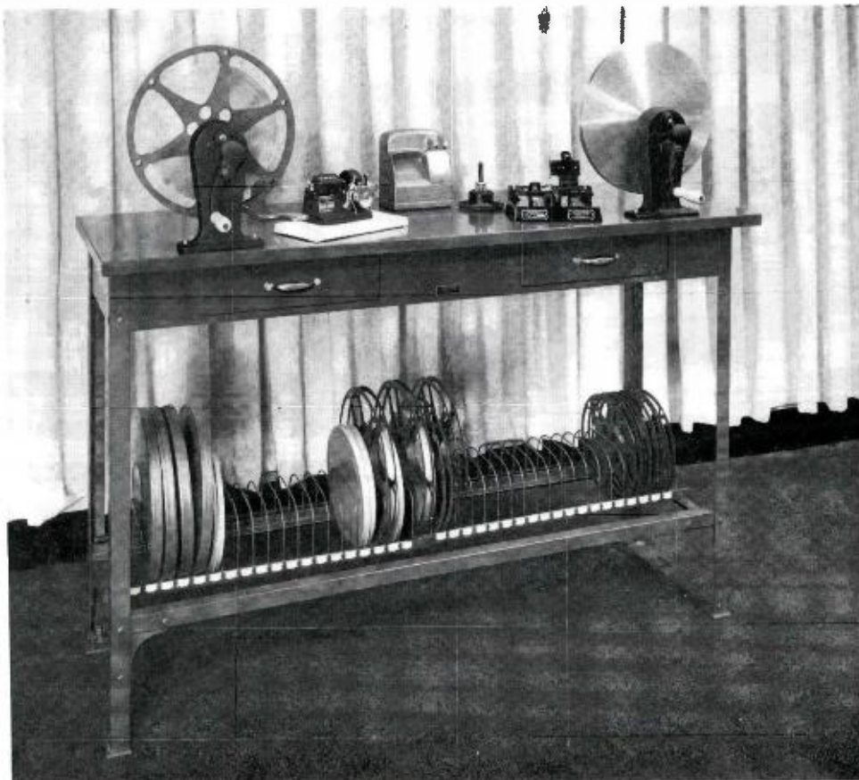
FIG. 1. View of a typical TV film editing bench setup for Television stations. Note that rewinds, splicer, viewer and measuring machine are needed.
