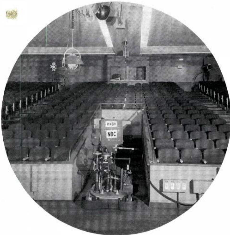
FIG. 1. Operating space of Studio D stage area includes this recess into audience seating area which allows movement of cameras for stage or audience shots.
