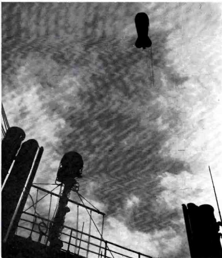
FIG. 2. This helium-filled balloon carries the antenna for the RCA 150-KW transmitter 1000 feet into the air.
