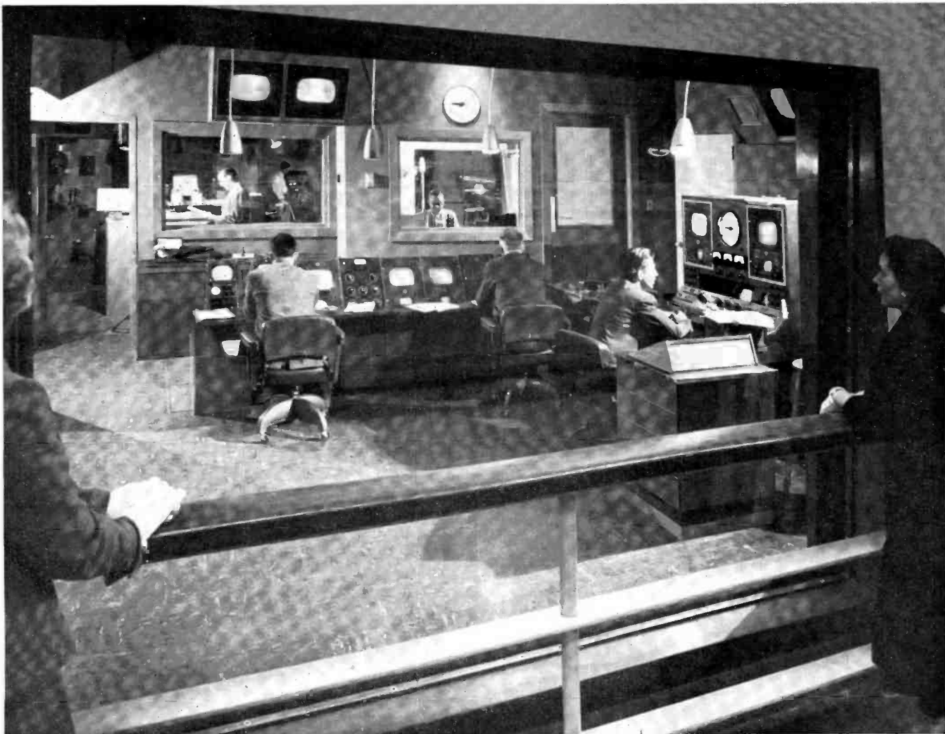
FIG. 38 (above). This is the WCAU TV Master Control Room as seen through the window from the main lobby. The film and announce camera monitoring positions are at the long console on the far side of the room. The master control switching console, especially built by RCA to WCAU's specifications is at the extreme right. The door at the left rear leads to the projection room, part of which can be seen through the window at the right of the door. The window further right looks into the announce booth, and through a second window into the part of the projection room where the announce cameras are located. The floor arrangement of this section of building is shown in Fig. 46.
