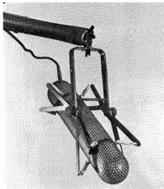
FIG. 4. Experimental highly directional gradient microphone—boom mounted—developed by Olson, Preston and Bleasley of RCA.
