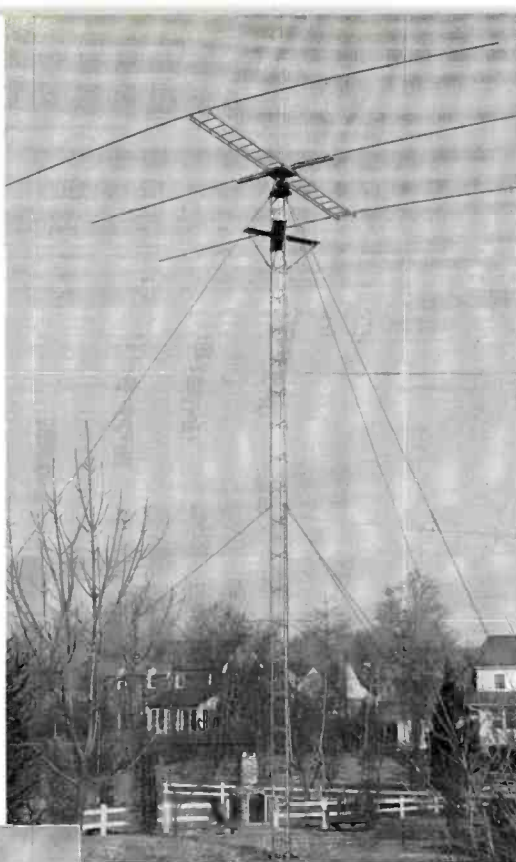
Bob's 20-meter rotary, perched on a 40-foot triangular tower, is inductively coupled to a low-impedance open-wire line.
