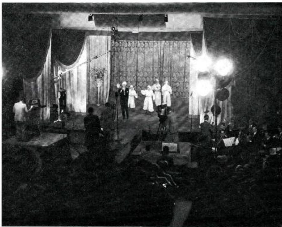
FIG. 16. Typical boom location in wings of an NBC-TV theatre.
