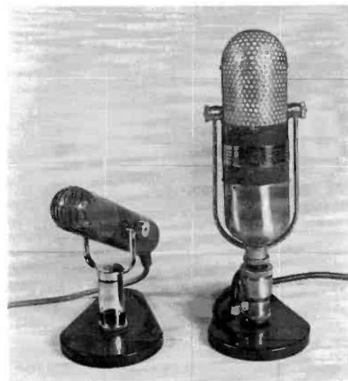
FIG. 13. Uniaxial microphone and the RCA 77-D as desk microphones.
