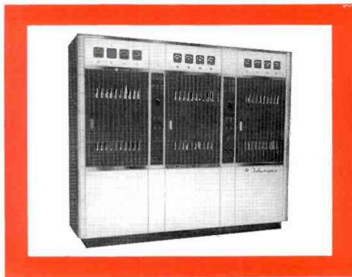
1-KW TYPE TTU-1B (FOR ERP* TO 27 KW). This transmitter and a UHF Pylon Antenna, can develop from 24 to 27 kw ERP on any channel, 14 to 83. TTU-1B is self-contained and all air-cooled. It is well suited as a driver for a high-power amplifier.
