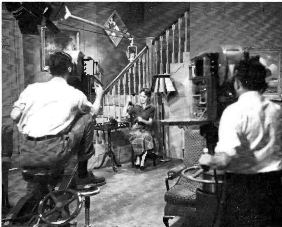
FIG. 6. Typical scene where boom must be raised rapidly from seated figure to rising position for wide angle pictures.
