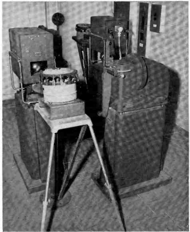
FIG. 14. Film room equipment consists of two RCA TK-20C film camera chains, two TP-2A Automatic Slide Projectors and two TP-9C Multiplexers.
