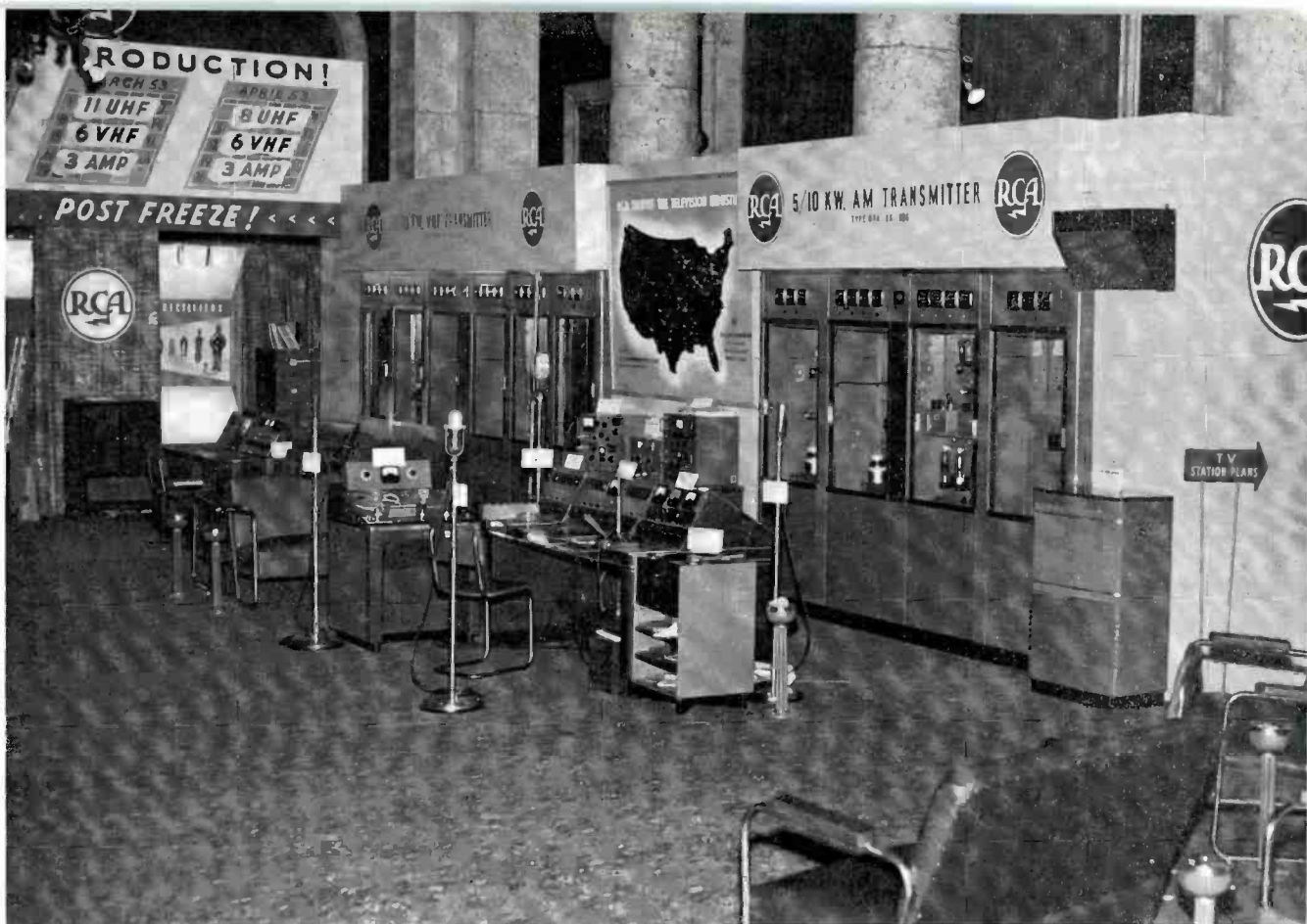
FIG. 3. The right wing of the RCA Exhibit featured two full-size transmitters—the new 10-KW VHF television transmitter, and the deluxe 5/10-KW AM transmitter—plus audio and control consoles, microphones and turntables.
