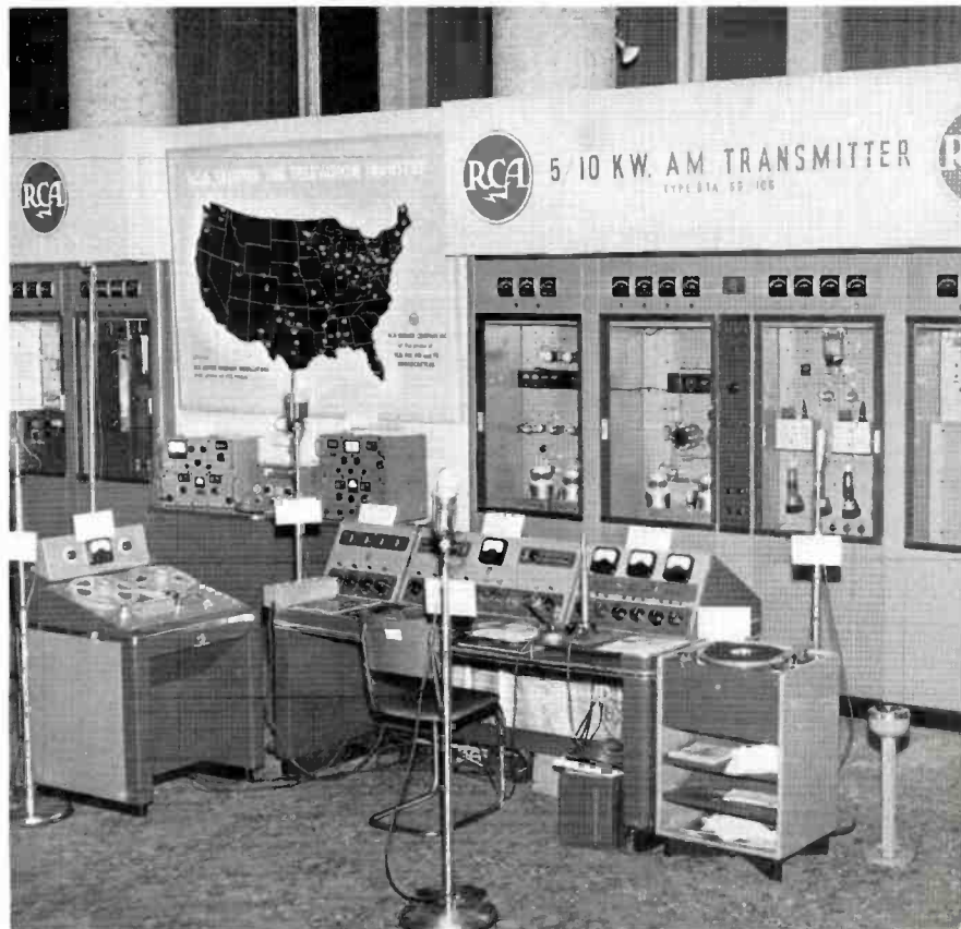
FIG. 7. A centralized group of AM audio and control equipment was located in front of the AM transmitter. At left of the console is the new tape recorder, and at right the new fine-groove turntable.
