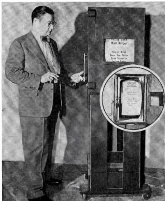
FIG. 10. A Studio Title Device: A mechanical method of creating a "crawl" title from the floor of a live studio. Prepared by the Graphics Section, the printed title is affixed to a specially constructed drum which is revolved on cue by manually- or motor-driven equipment.
