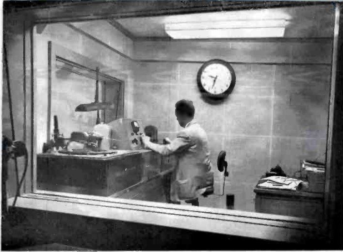
FIG. 11. The recording room with 73-B professional recorder. A 50-watt McIntosh amplifier drives the recording heads which is so flexible it can record from 20 monitoring busses.
