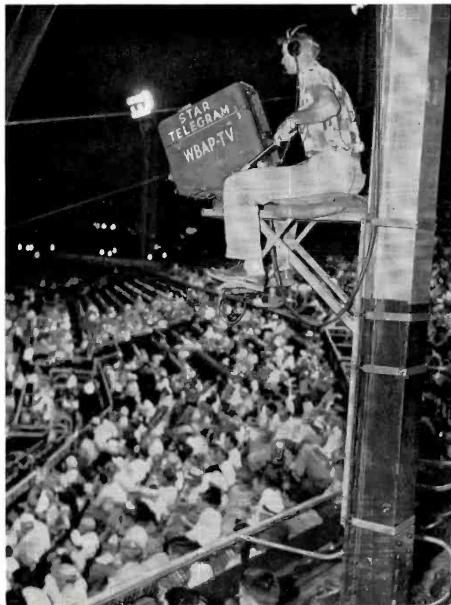
FIG. 26 (below). To improve their baseball pickup (cameras in press box were too high) WBAP engineers rigged up this "cowboy camera" in the Ft. Worth ball park.
