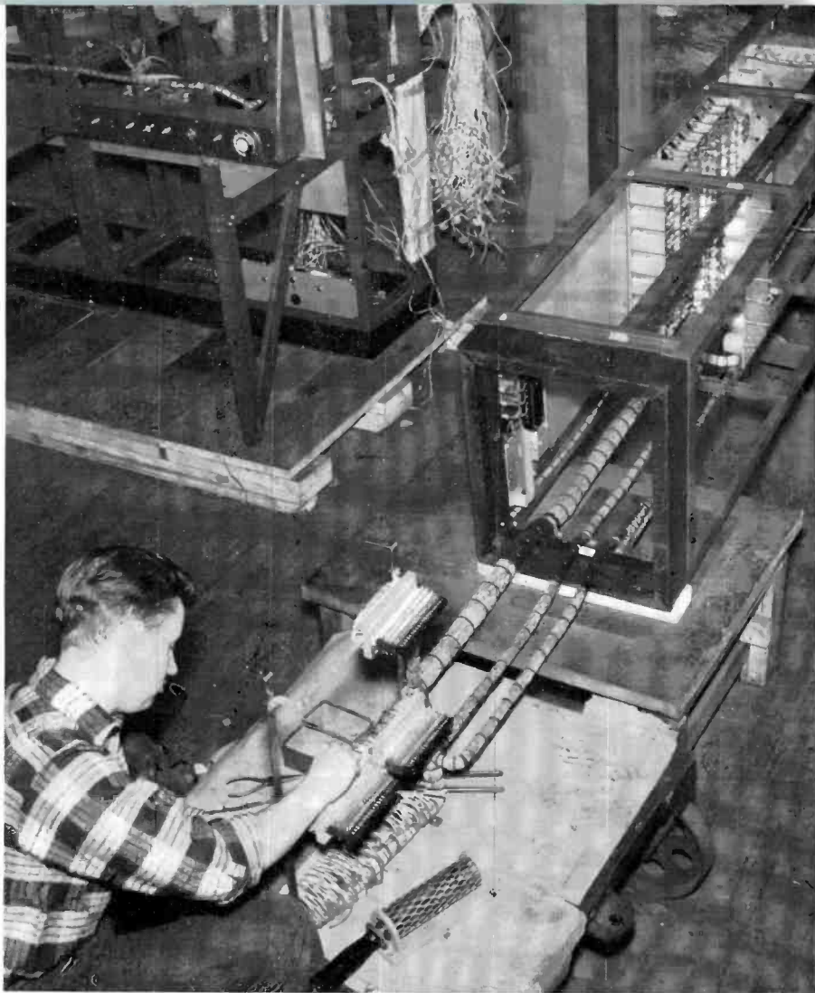
FIG. 2 (right). All of the WBAP racks were wired in the RCA plant at Camden. Cables to terminal boards were made about three feet longer than usual. After racks were set in place at WBAP the terminal boards were dropped through holes in the floor and mounted on a frame in the basement as shown in Fig. 1.
