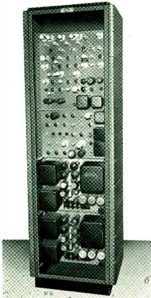
FIG. 8. View of the Vidicon power supplies and amplifier units which are rack mounted for convenience.
