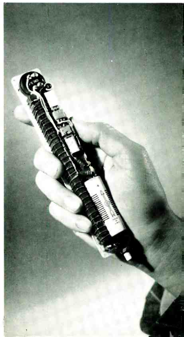
FIG. 7. A cigar-size experimental microphone-transmitter, modulated by a tiny built-in dynamic microphone. Employs two developmental junction type transistors, coil and battery.
