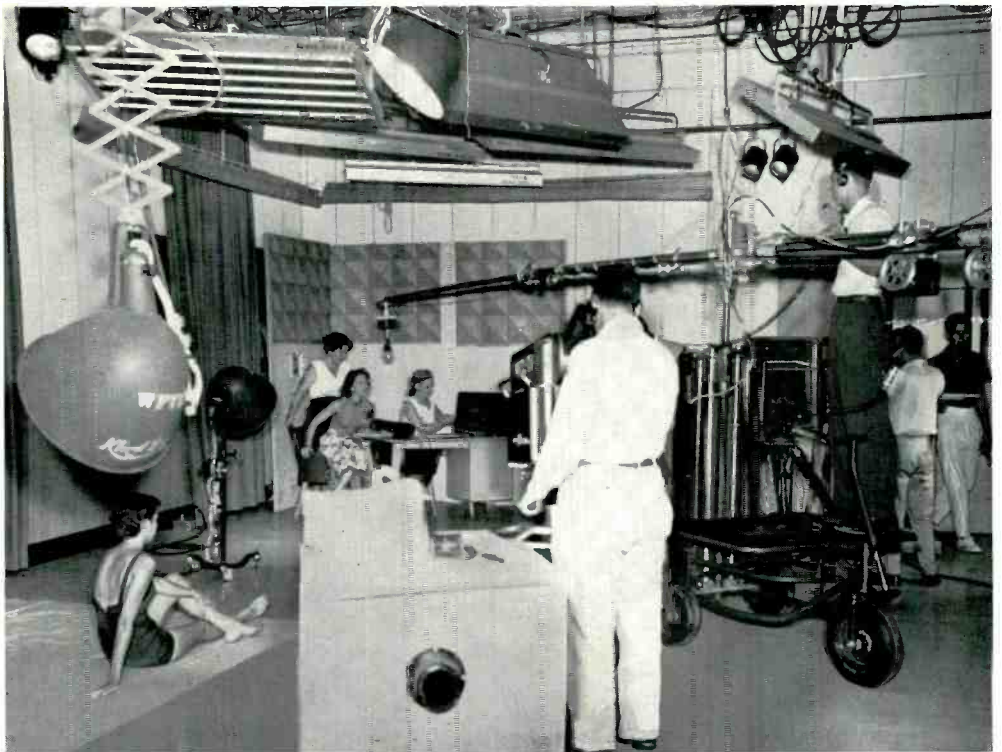
FIG. 2. "On-the-Air" shot in main arena studio portrays vivid view of operational layout. RCA Boom and Perambulator supports TV-famous 77-D microphone.
