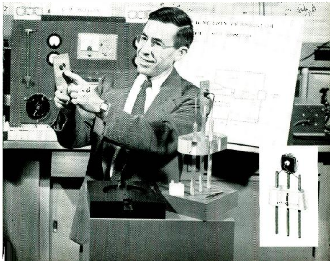
FIG. 24. Dr. C. W. Mueller of the research staff of the David Sarnoff Research Center of RCA Princeton, N. J., points to a "blown-up" model of the heart of an RCA developmental junction-type transistor. Complete interior model is seen at right. A "p-n-p" junction-type transistor is shown in the inset at lower right.
