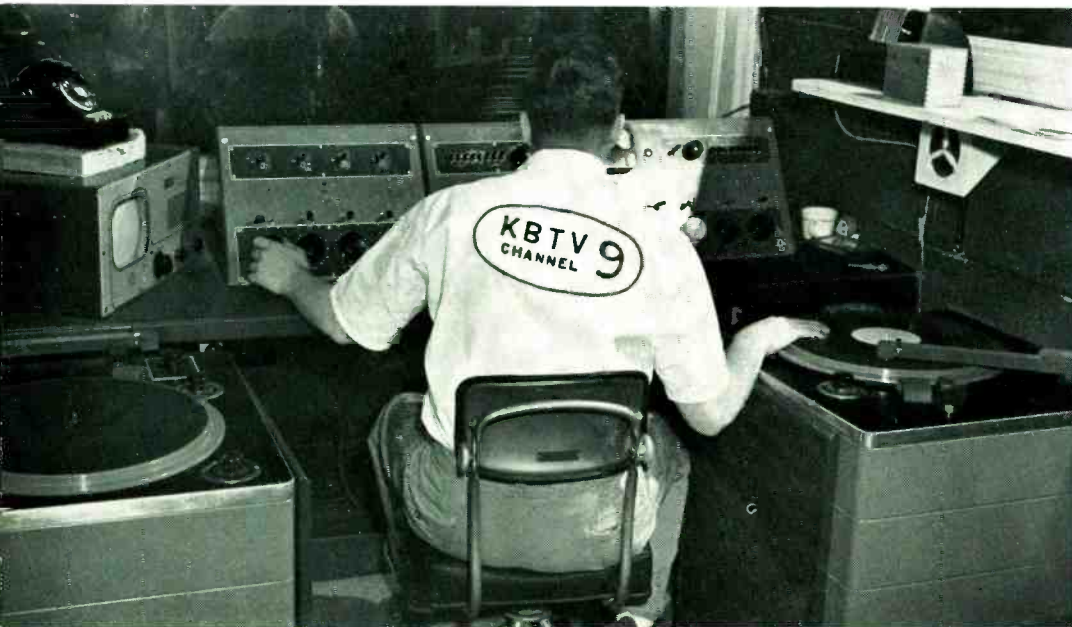
FIG. 5. KBTv's compact yet highly efficient Audio Control area where the audio engineer controls all sound going out over the air.
