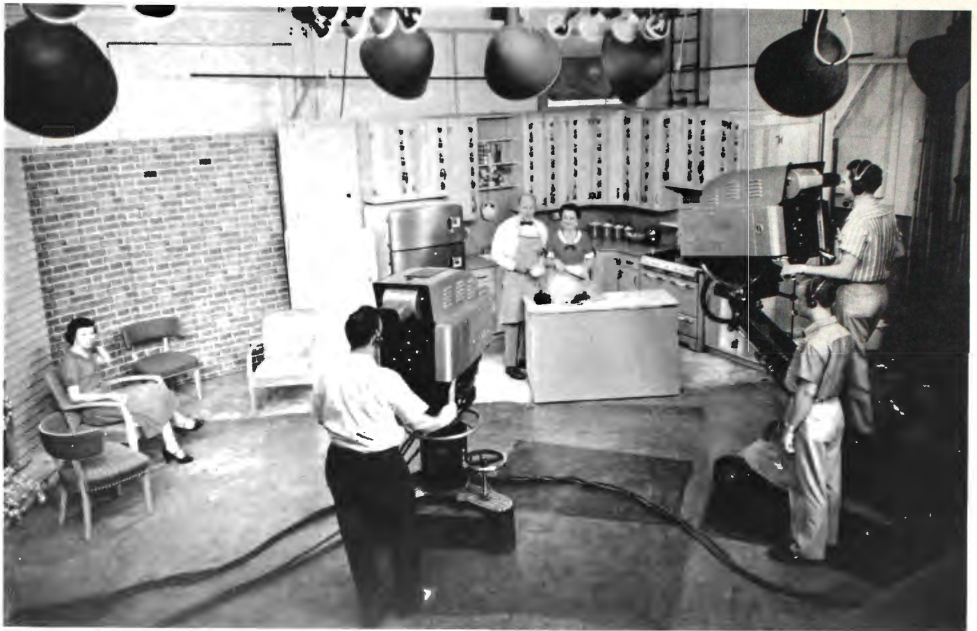
FIG. 33. WBAP-TV studio scene showing a typical color telecast. Note that the color cameras are used with standard type equipment such as two-man dolly and lighting equipment. Cooking demonstrations are in kitchen and interviews are held at left part of set.
