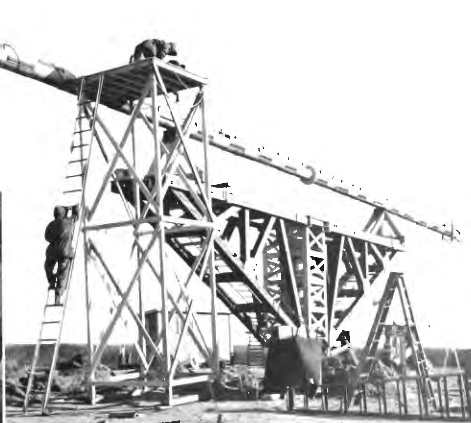
RCA engineers inspect the flanged joint at which the two sections of the ultragrain antenna have been assembled prior to hoisting the antenna on top of the turntable for pattern and gain measurements.
