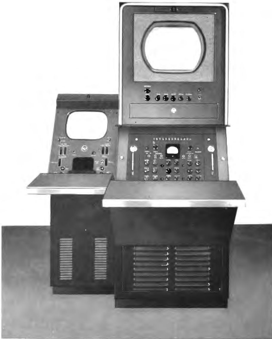
FIG. 16 (left). The complete 3-V Camera Control equipment includes a TM-6C Monochrome Monitor, a 19-inch Console containing the camera control panel and processing amplifier and a Type TM-10B Color Monitor. These three units may be grouped together as shown here. Or the color monitor may be suspended from the wall or ceiling for better visibility (by producer, technical director, etc.). The two console units can be located separate from the monochrome control units or mounted in line with them. When desired the control panels can be furnished for rack mounting as shown in Fig. 28, page 51.
