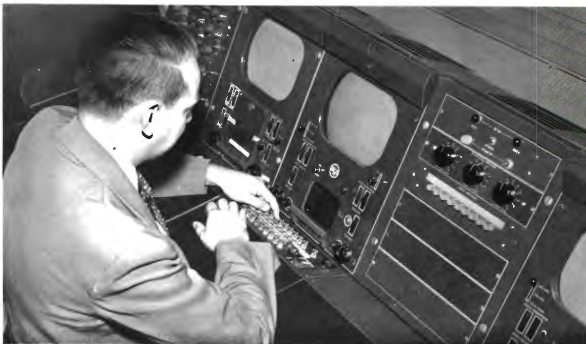
FIG. 29. View of the new TS-11A Video Switching Panel shown mounted in the sloping desk section of a typical Control Console. The TS-11A provides 9 inputs and 3 rows of push buttons for fades, lap dissolves and super-positions.
