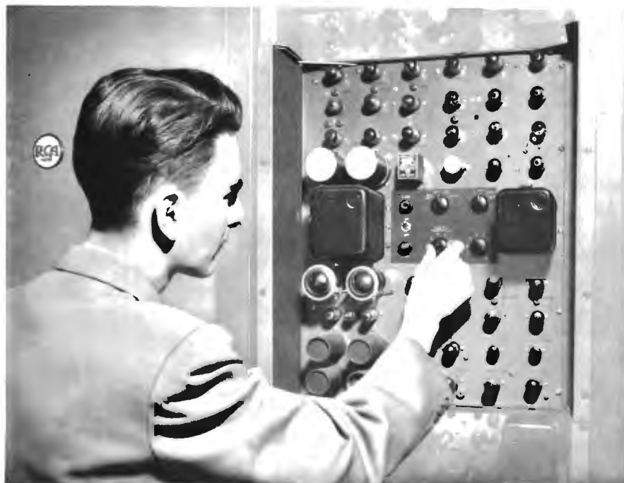
FIG. 9. View of the advanced design Sync Generator which has reduced the rack space to one-third that occupied by former designs. Providing extra stability, small size and combining all sync functions in a single chassis, it is ideal for color TV applications. It includes a built-in Genlock, dot generator, grating generator and regulated power supply.
