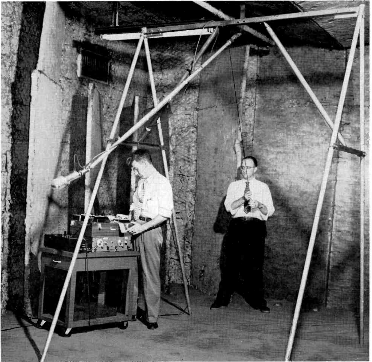
FIG. 1. Producing a standard, controllable quiet wind by use of a pendulum device in the transducer design laboratories at the RCA Camden Plant.
