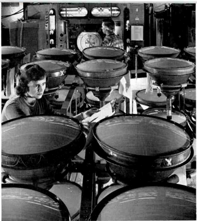
FIG. 8 (right). RCA 21-inch color kinescopes approach the end of a production line at the plant in Lancaster. At the final test position each tube receives an operating check.
