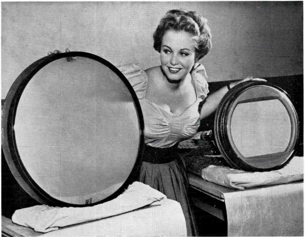
FIG. 1. The RCA 21-inch color television picture tube, left, is shown here in comparison with the 15-inch color tube with which RCA launched commercial production of color TV in March 1954. The 21-inch color tube utilizes the same operating principles as those of the previous RCA color kinescopes. It is a shadow-mask design employing a three-beam gun. An important feature is the thermally compensated formed shadow mask. It has a deflection angle of 70 degrees which permits an increased picture area with short tube length. In addition, it uses phosphors on the faceplate of the tube, a metal envelope, and a short electromagnetically converged gun.
