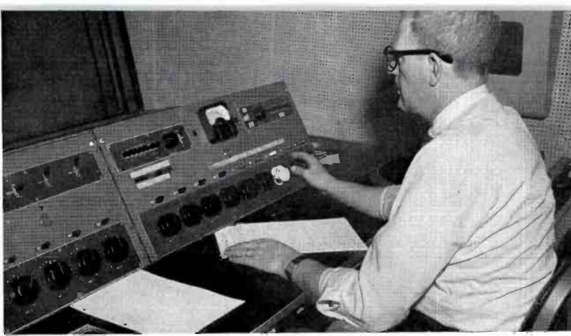
FIG. 20. Remote control video buttons installed on BC-2B audio console permit one-man audio/video switching.
