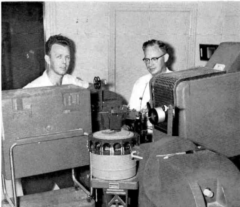
Lee Hunt, film director (left), and Leon Nolan, chief photographer (right), examining the process of feeding four picture sources into an iconoscope camera chain.
