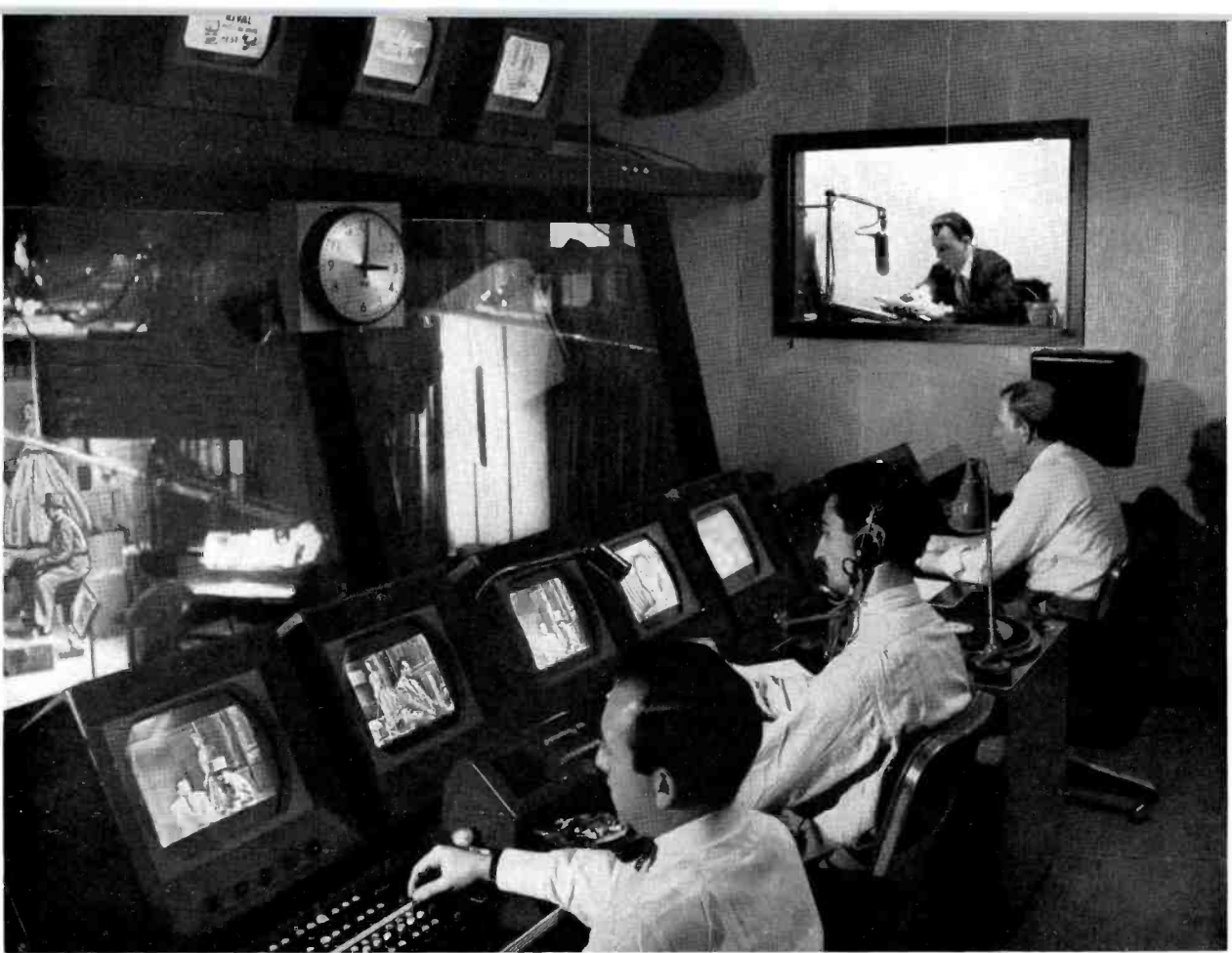
FIG. 14. Studio 11 control room in action. Left to right are video switcher, director, audioman and announcer. Camera control operator sits farther to left (not shown).
