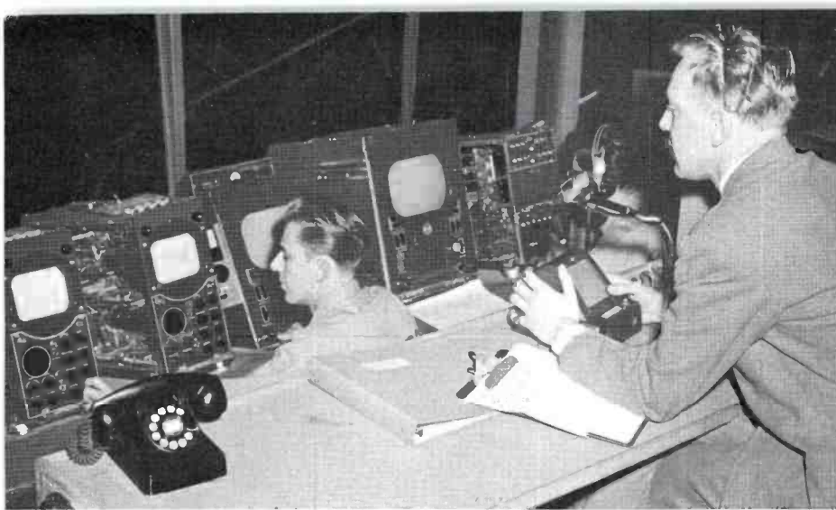
FIG. 18. View of control room showing video equipment—two field camera controls, auxiliary switcher, film camera control, master monitor and field switcher. Operators Carl Johnson (left) and Frank Muriel.
