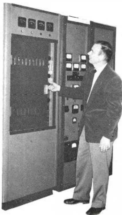
FIG. 6. Anthony F. Hogg, Chief Engineer, observes meter readings on the AM transmitter. Mr. Hogg keeps station operating at peak efficiency as proved by a recent nationwide Conelrad alert. WHLM, key Conelrad station in Bloomsburg area, made switch from 550 to 640 kc in 30 seconds.
