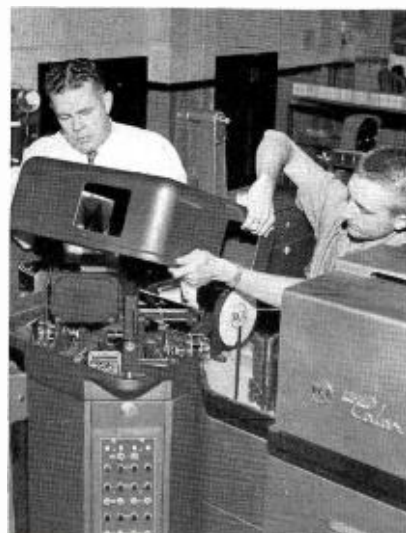
FIG. 2. Final check is made on 3-V color film chain multiplexer. An input for opaques has also been provided in this equipment.
