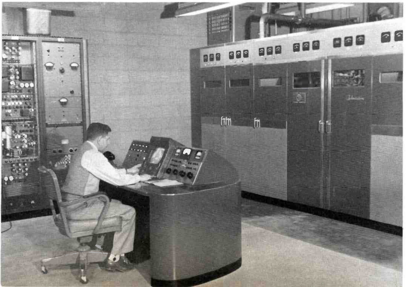
FIG. 10. RCA TT-5A transmitter showing input equipment. Earl Nelson operator.
