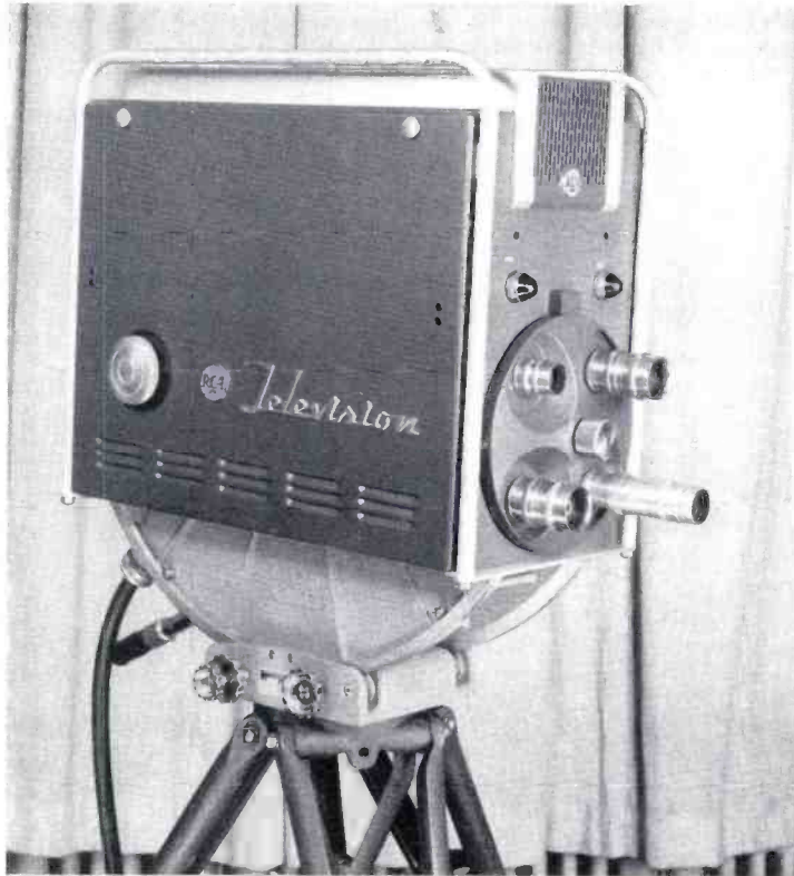
FIG. 1. Vidicon Studio Camera. Type TK-15. offers operating economy of the vidicon tube in a camera designed to broadcast standards. This new camera features a built-in 7 inch viewfinder and 4-lens turret for broadcast operations.
