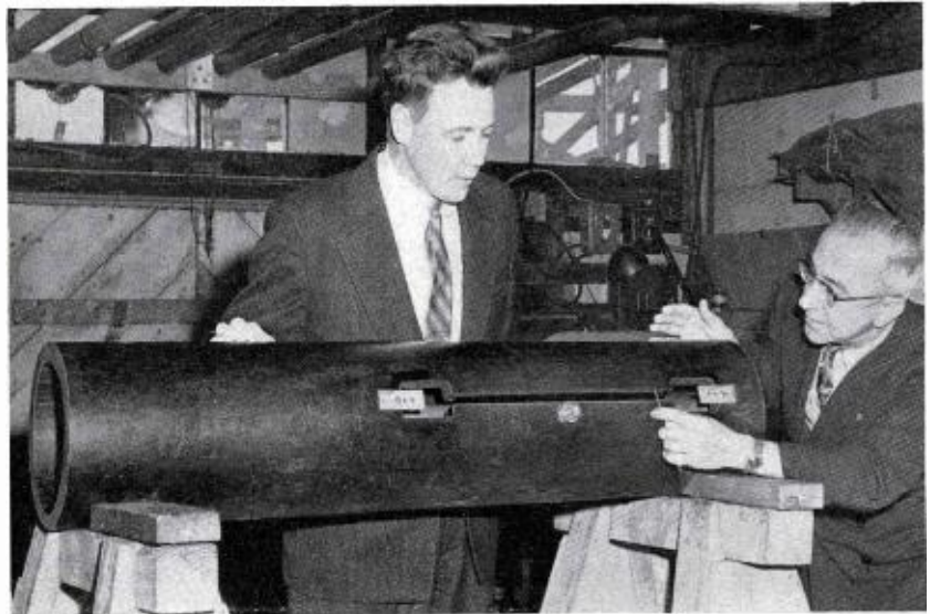
FIG. 7. Final inductively tuned slots for a gain of 9 antenna on 10 3/4 inch diameter pole section being inspected by the authors, Matti S. Siukola (left) and George A. Kumpf.
