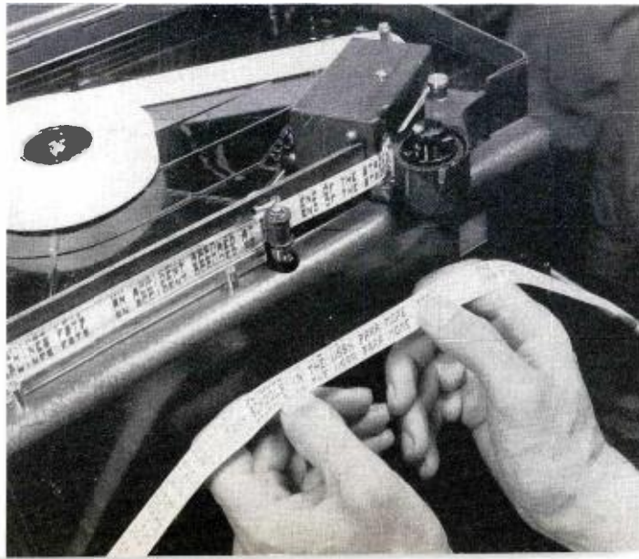
FIG. 21. Typical output of a Hellschreiber recorder. This is being fed from an RCA Communications receiver. The monitoring output at Schleissheim is fed to Munich via telephone lines.
