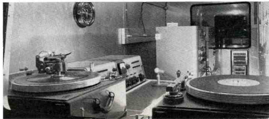
FIG. 4. Original RFE radio studio and control room on wheels, in Germany. It occupied one tractor of the seven-tractor broadcast station.
