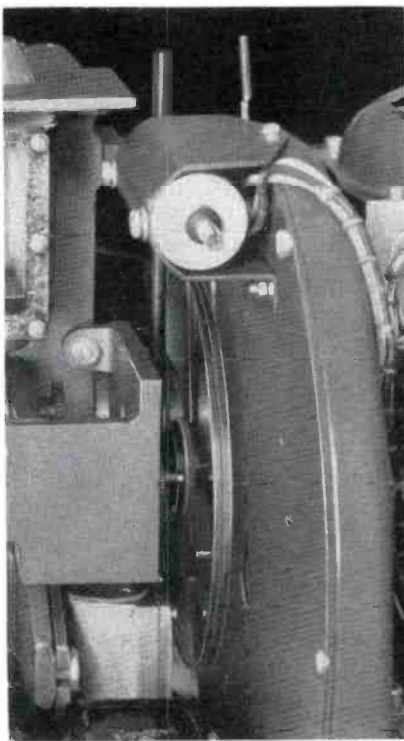
FIG. 9. Neutral density disk video control built into 16mm motion picture film projector.
