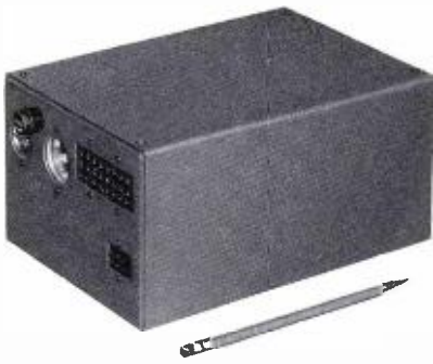
FIG. 13. Compact auxiliary control box houses all relays, drum and mirror motor capacitors.
