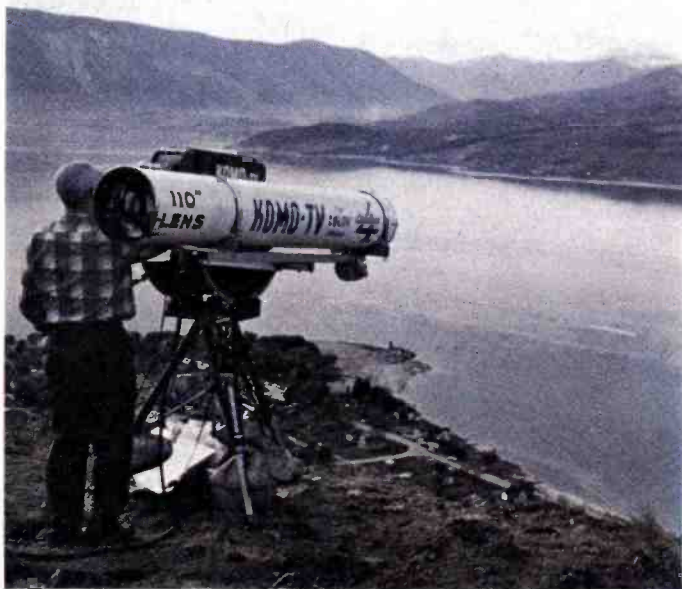
FIG. 29. Giant 110-inch sports lens in use at annual hydroplane race on Lake Chelan. This gives viewers a close-up of all action. At a distance of one mile this lens can close down on a man in the cockpit of the boat.
