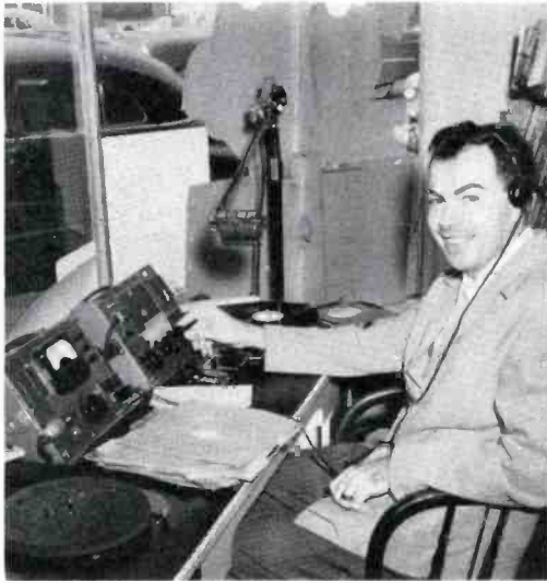
FIG. 8. OP-6/OP-7 Remote Pickup Equipment is used to originate d-j programs from local stores.
