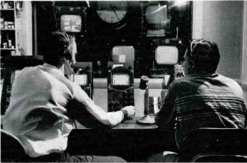
FIG. 19. Studio B-C control room with T.D. Fred Fowler at the black-and-white camera controls and Director Ed Lackner at the studio switcher. All black and white live camera equipment at the studios (a total of four chains), is of the field type, thereby, allowing it to be transported into the field for use on remotes as necessary.
