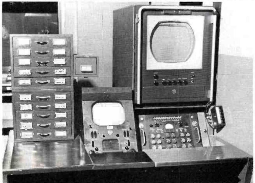
FIG. 17. This is control position of 3-V Color Film System. Note cabinet at left, used for filing of all currently operational 35mm slides. The push-button switch at lower right controls the input to the TM-10B Color Monitor. This monitor can be switched to either incoming Network, Line out to transmitter, Studio B-C, or the 3-V Color Film Camera.
