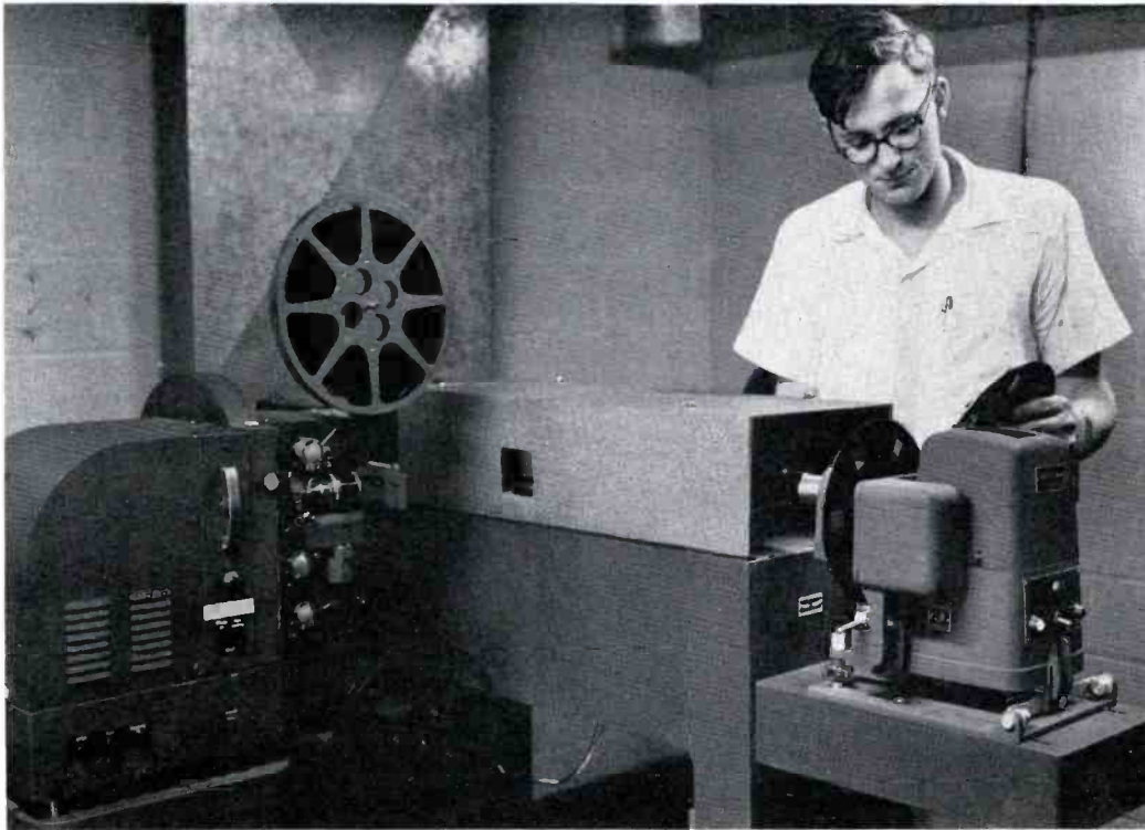
FIG. 46. Taylor Rogers, WUNC-TV Transmitter Engineer, at film and slide chains located at transmitter site.
