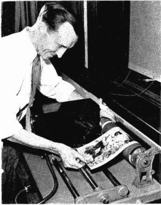
PRINCIPAL ELEMENTS OF THE MODERN RADIOPHOTO SYSTEM ARE THE ROTATING CYLINDER, THE LEAD SCREW (CENTER ROD OF THE THREE) AND THE SCANNING OR RECORDING HEAD IN THE BLACK BOX.
