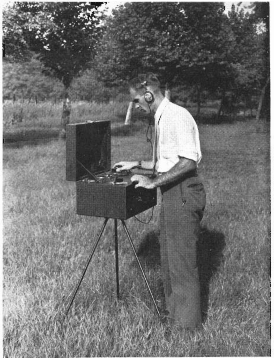
FIG. 4. NEW TYPE TMU-21 FIELD INTENSITY METER BEING USED IN THE FIELD BY MR. GIHRING, RCA VICTOR ENGINEER. NOTE COMPACTNESS AND CONVENIENT TRIPOD MOUNTING.
