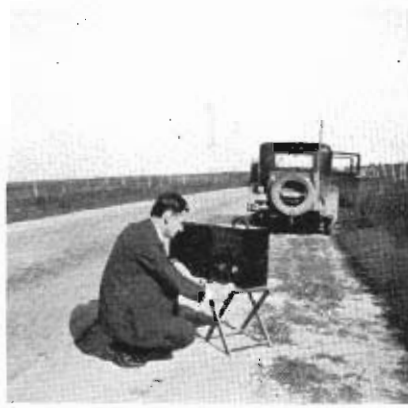
FIG. 3. CUMBERSOME OLD-STYLE FIELD INTENSITY MEASURING EQUIPMENT BEING USED BY MR. ADLER, RCA VICTOR SALES ENGINEER, OCTOBER 1930.
