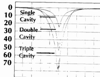
Response of single, double and triple cavity notches with same 3 dB bandwidth.
