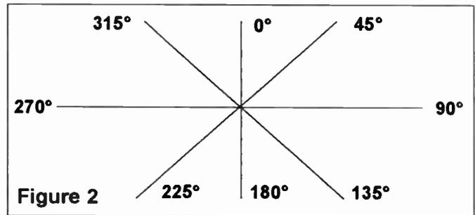
At this point we take the height above sea level of the antenna site, add to it the height of the antenna, then subtract the average of the eight radials. This yields what is known as Height Above Average Terrain.
