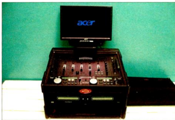
A portable "DJ Pod" remote may be used as an emergency studio set up.
