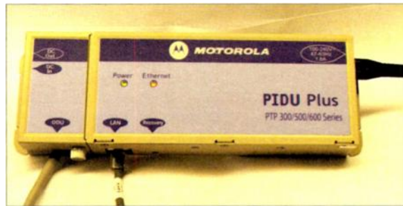
The Motorola “In Door Unit”
