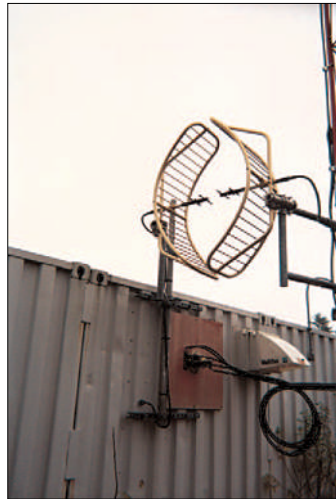
Two Mini-Flectors were used to create an "isocoupler."
