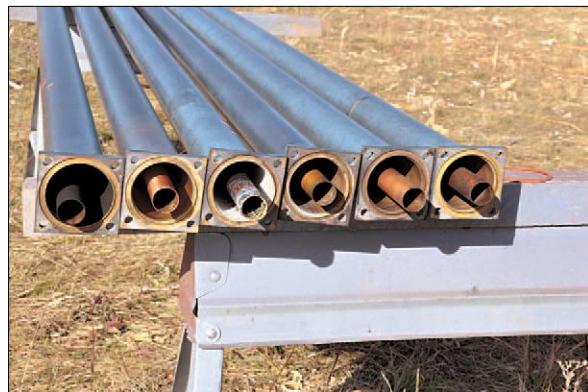
Note the extreme damage on the 3rd from the left inter-bay section.
