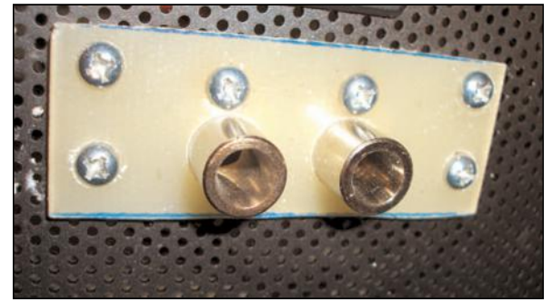
Mounted speaker jacks note they are isolated from the metal panel by an insulated material
