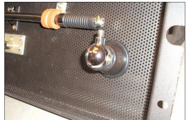
The antenna dipole mounted for transport and the silver ball antenna mount for use.
