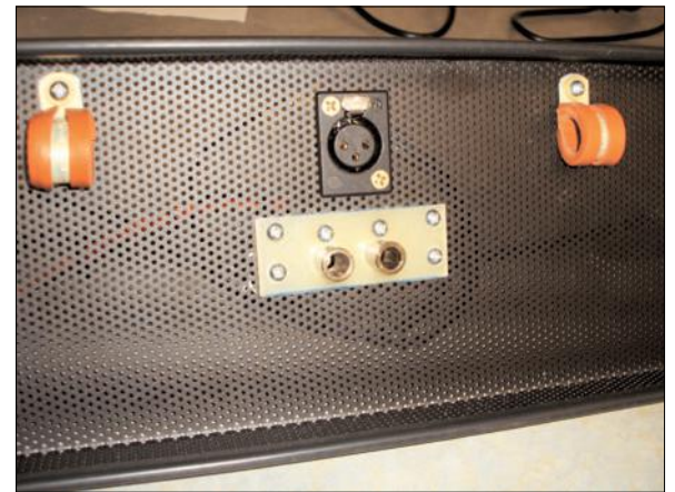
The rear panel showing the IFB port, jacks and the holders or the dipole when not in use
