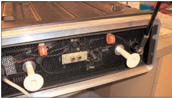
PA rear showing completed unit including AC cord spools, all jacks and deployed dipole.
