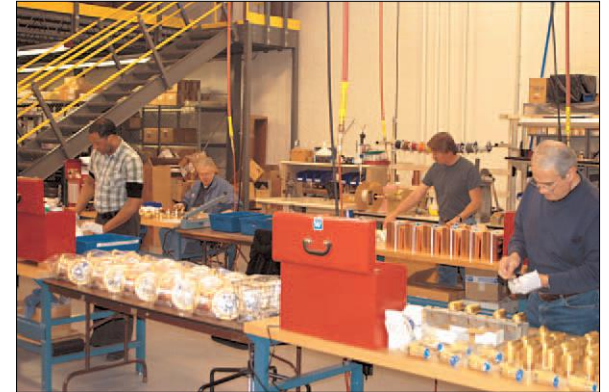
Myat employees assembling elbows and reducers.
