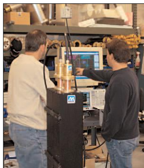
Tuning a cavity filter at Myat's factory.
