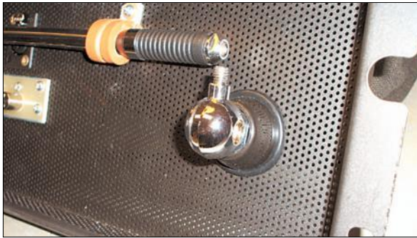
The antenna mounted on the rear panel.
