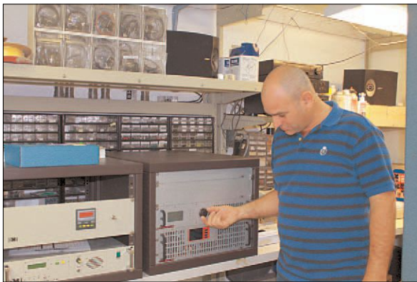
OMB USA technician Victor Cabrera, changing frequency on a transmitter in test.
