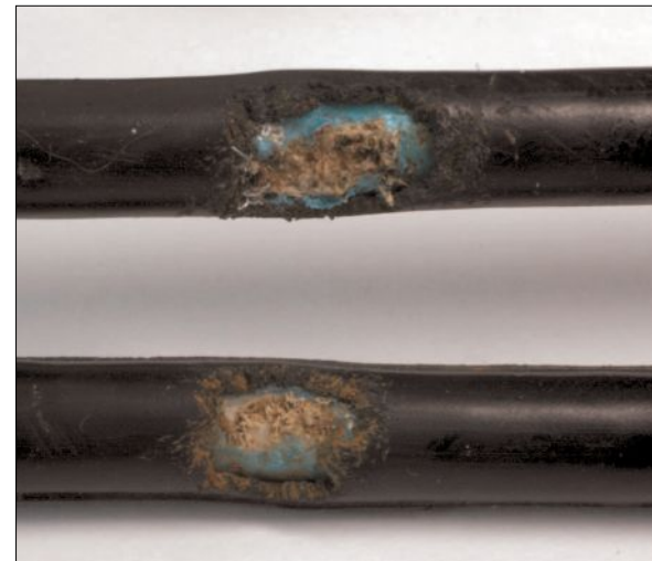
Fig. 5 – Varmint-induced impedance discontinuities.
