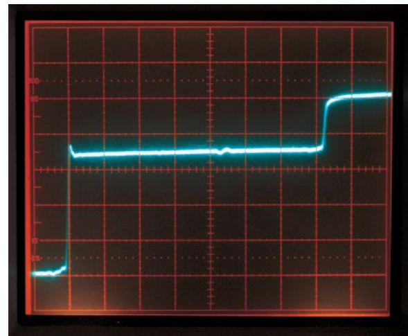
Fig. 2 – Measuring the velocity factor of RG/6.
