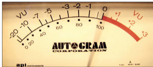
An average level VU meter will not show the audio peaks.
