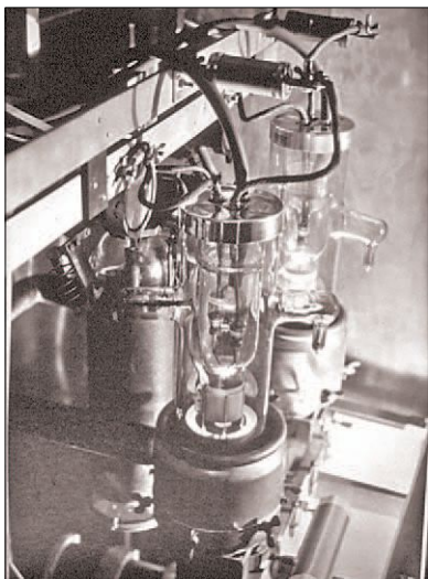
WLW power tubes in cooling cylinders.
