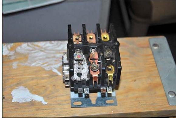
K3 Disintegrated Contact
