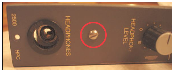
Figure 1 – Grounding Screw Installed
