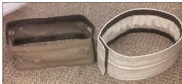
Original Harris FM25K air duct on the left and replacement air duct on the right.
