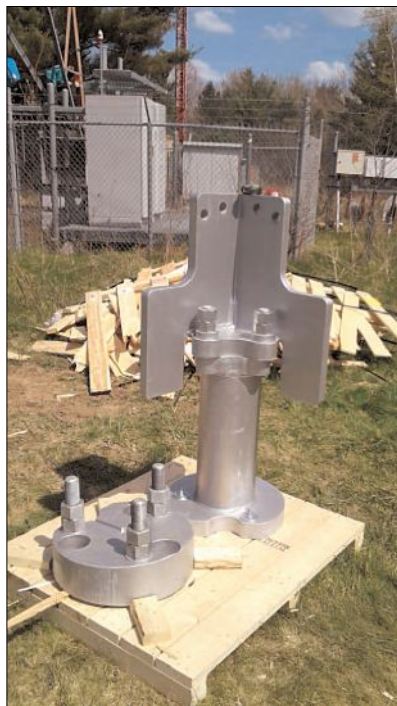
Steel Pedestals Replace Insulators
