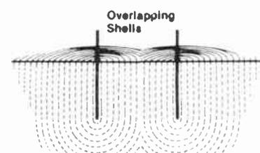
Figure 6. Minimum Resistance Obtainable with Parallel Rods in a Square of Given Area.
