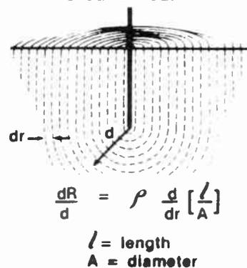
Figure 3. The Influence of Ground Rod Physical Parameters
