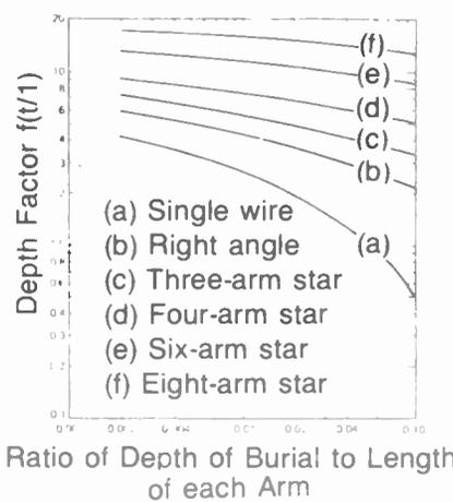
Figure 10. Self Inductance of Grounding Wires
