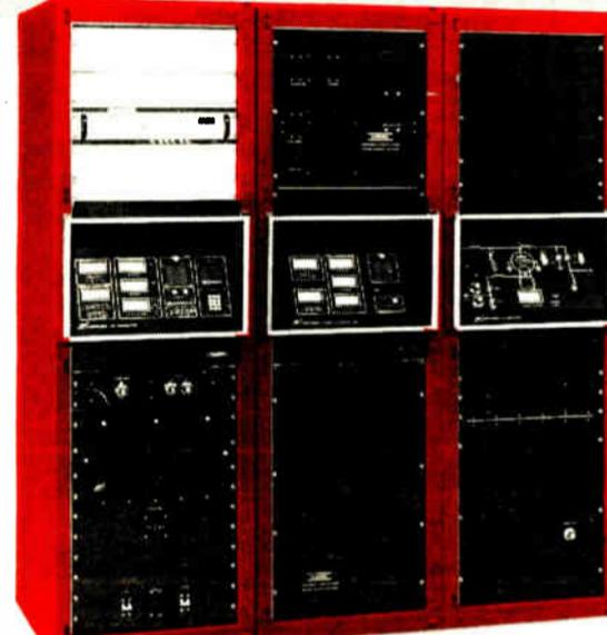
Case in point: Our new 20/30KW FM Transmitter. One of the QEI "New Reliables." Everything about it is designed for maximum efficiency and ultra-dependability. Its single tube design uses a grounded grid triode for greater stability.
