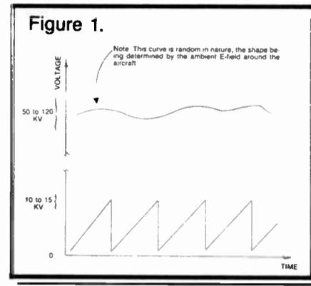
when the sharp points cause ionization of the surrounding air, instantaneously discharge the capacitance of the aircraft after which the aircraft will then recharge and the cycle is repeated (Reference 1).
