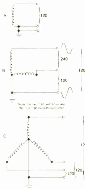
Figure 2. Capacitive coupling between power transformer and ground can cause leakage currents to flow in a system with audio equipment powered from out of phase AC lines.
