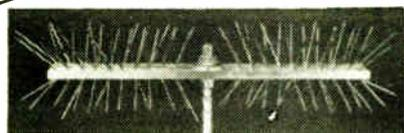
Through the use of sharp, stainless steel points, the Stati-Cat System provides a continuous low-resistance discharge path for the static electric charge found on all tall structures. Charge dissipation prevents the high voltage gradient between cloud and earth that eventually leads to the sudden massive discharge known as lightning.
