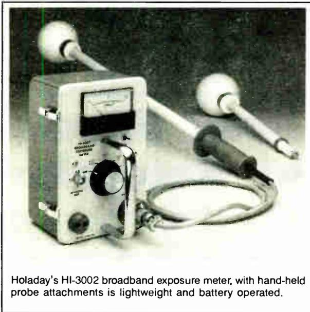
Holiday's HI-3002 broadband exposure meter, with hand-held probe attachments is lightweight and battery operated.
