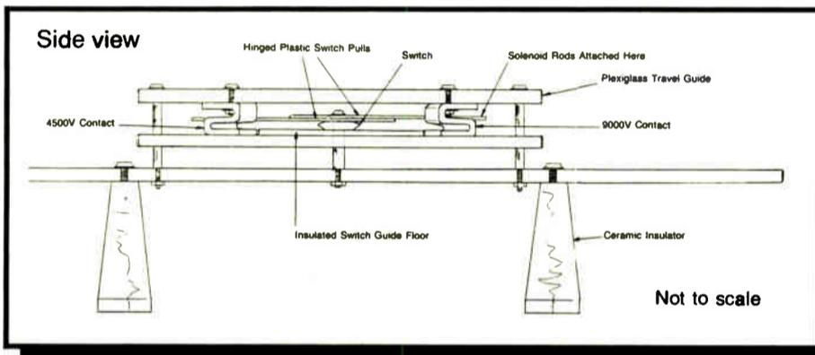
An ideal material to use for the pulls are the plastic engravers used to make "No Smoking" signs. A good solenoid to use is something like a Guardian LT8x16 for continuous duty.
