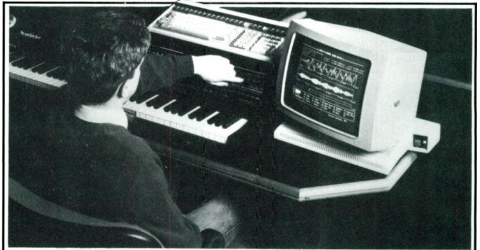
New England Digital's Synclavier integrates a piano-type keyboard into its workstation design.
