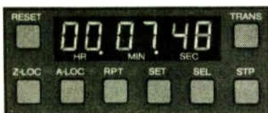
**Motion-sensing transport control** for safe, smooth tape handling.
