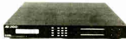
The AD2100 provides from 0 to 5.4 seconds of stereo audio delay (10.8 sec. monaural) for talk show censoring, lip-sync error correction, or to compensate for video processing delays. Delay can be set manually, or controlled by a frame sync. standards converter or other device for automatic delay tracking.
