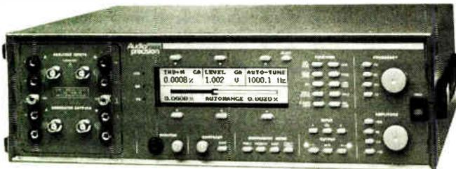
The generator provides transformer coupled outputs with a frequency range of 10 Hz to 120 kHz, up to 26 Vrms, and balanced/unbalanced configurations. The dual channel analyzer provides 250 Vrms input, 1.5  $\mu$ V residual noise, residual distortion below 0.0025 percent and frequency range of 10 Hz to 300 kHz. Combined generator and analyzer amplitude accuracy is  $\pm 0.2$  dB with frequency response flatness of  $\pm 0.05$  dB from 20 Hz to
