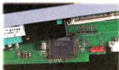
Our proprietary gate array logic generates both module control and remote control of connected equipment.
