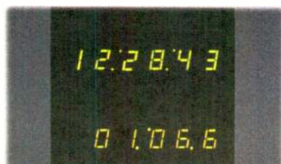
The digital timer displays the tenth of second digit in the Hold and Stop modes, but blanks it when time is running to minimize distraction to the board operator.
