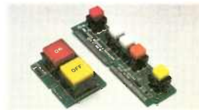
Sealed, LED illuminated buttons are designed so you can remove the switch assembly without unsoldering, in case of a coffee spill.
