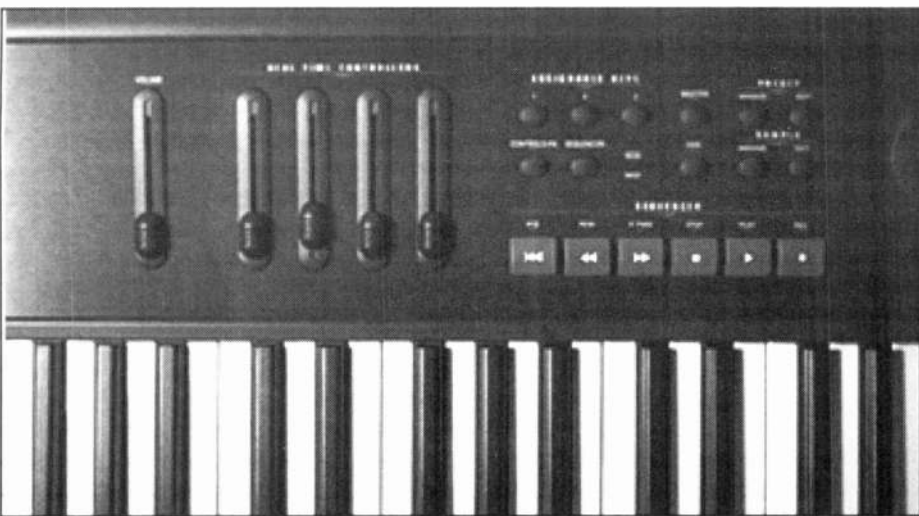
Sliders to the left are the Real Time controllers. Edit and disk access buttons are shown above the rectangular Sequencer keys.
