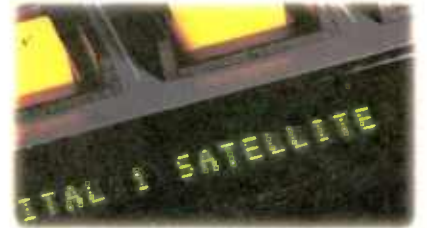
Each fader has a 10-character alphanumeric display. The display changes when another audio source is assigned, which can happen either manually or at a preassigned time.
