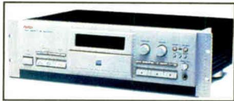
The CR200 is a stand-alone recording unit with XLR balanced +4 dBu inputs, AES/EBU connections and RCA -10 dBv jacks. An internal sample rate converter accommodates any digital input signal from 32 to 48 kHz and converts it directly to the CD standard of 44.1 kHz.
