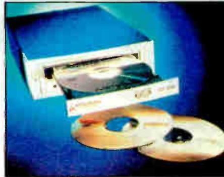
the SCSI interface and includes a 1 MB buffer to prevent data transfer underruns.
