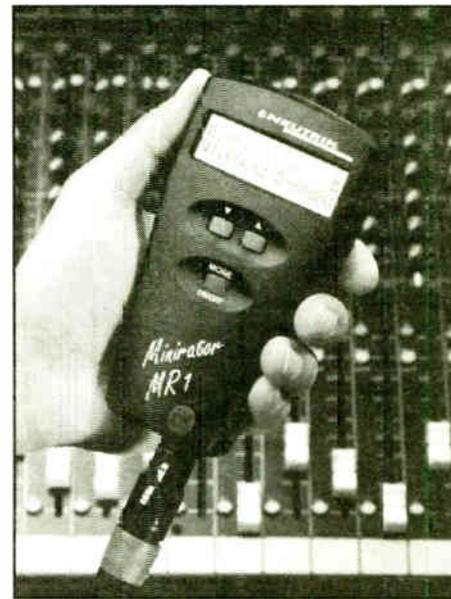
The Neutrik MiniRator MR-1 features three-button operation and balanced output.
