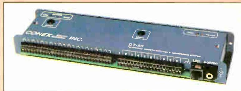
then allows remote control of 10 SPDT relays as well as the remote monitoring of 10 external switch contacts or logic levels. Status lights indicate ringing signal, power, DTMF tone detection, line connection, and access.
