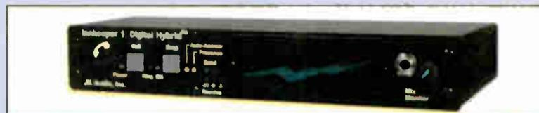
cross talk common to analog hybrids. The DSP continuously monitors both the phone line and audio signals to deliver separation.
