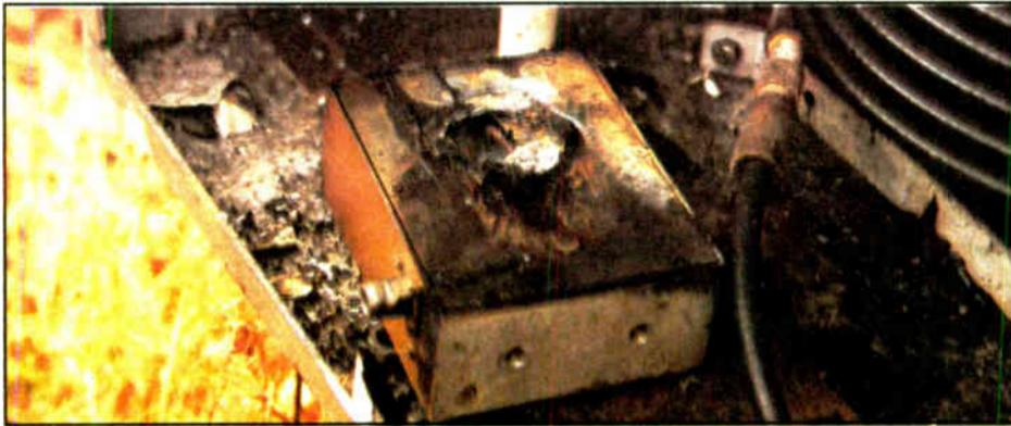
Figure 5: This toroid was damaged by lightning.
