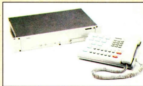
interface to six telephone lines and is expandable to 12 lines. The dual hybrids allow the TS612 to operate as a single-studio telephone system able to conference up to four callers simultaneously or as a two studio system able to
