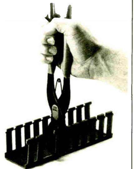
The company says the tool is ideal for use on its Panduit Type G and E Slotted Wall Duct and that it easily cuts two-inch-tall fingers. Taller pieces can be removed in multiple "bites."
