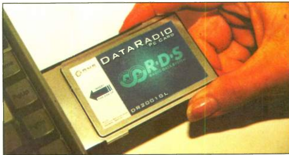
Personal Computer Memory Card allows RDS Data to be displayed on laptops.
