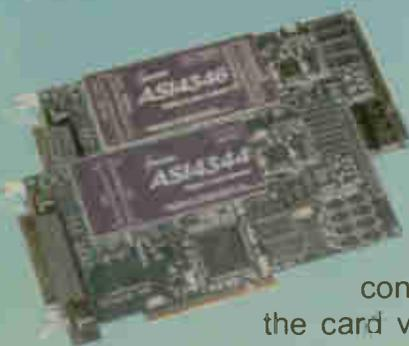
This is the first time a professional audio company has created devices specifically for the MP3 format. The two cards decompress audio files on their own hardware so the processor doesn't have to. With these cards, the skipping and slowness that plague broadcasters with MP3 files have been eliminated.
