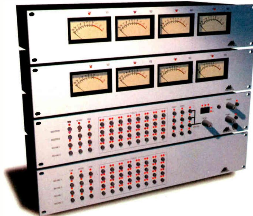
Master and slave panels communicate via serial connections, permitting distributed placement and allowing multiple master panels. Serial control permits the use of a roving control panel to allow the controls to be near a particular source. Store button can be used to save up to 32 snapshots of source, meter and speaker outputs. Store also will save oscillator frequencies and levels from the digital sinewave oscillator and pink noise generator.
