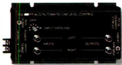
The FP-ALC2 (shown) is the stereo version, with phono jack I/O. The automatic level control circuitry maintains a consistent -10 dBV output for input signal variations as great as 25 dB.
