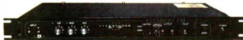
Bass enhance allows the unit to be tailored to any format with the adjustment of one control. Broadcast Technology's "smart clipper" enhancement increases loudness of the audio without creating excessive distortion. It looks at the audio and determines if clipping or limiting is appropriate.
