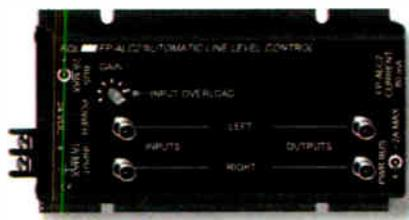
The FP-ALC2 (shown) is the stereo version, with phono jack I/O. The automatic level control circuitry maintains a consistent -10 dBV output for input signal variations as great as 25 dB.
