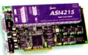
Need analog today but digital tomorrow? The multi-stream ASI4215 sound card from AudioScience has both. It combines the flexibility of independent sample rates and compression formats with a choice of balanced analog and AES/EBU or S/PDIF digital I/O. Combine this with DSP based MPEG compression for minimal CPU loading and maximum responsiveness. With the ASI4215, your station automation system is ready for action, now or in the future.
