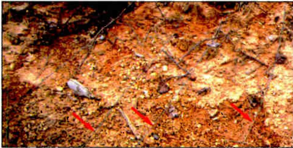
Fig. 1: Rain can erode soil and expose ground radials.
