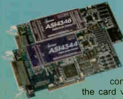
This is the first time a professional audio company has created devices specifically for the MP3 format. The two cards decompress audio files on their own hardware so the processor doesn't have to. With these cards, the skipping and slowness that plague broadcasters with MP3 files have been eliminated.
