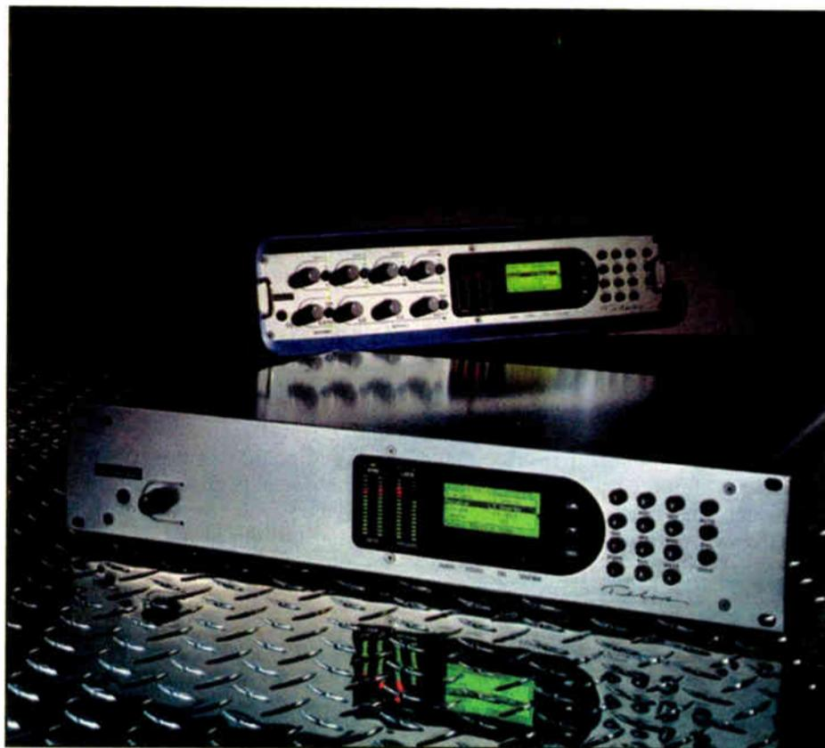
With the Xstream, however, it's also possible to receive 15-kHz audio from two separate locations — particularly useful when contributions are needed from several outside sources.
