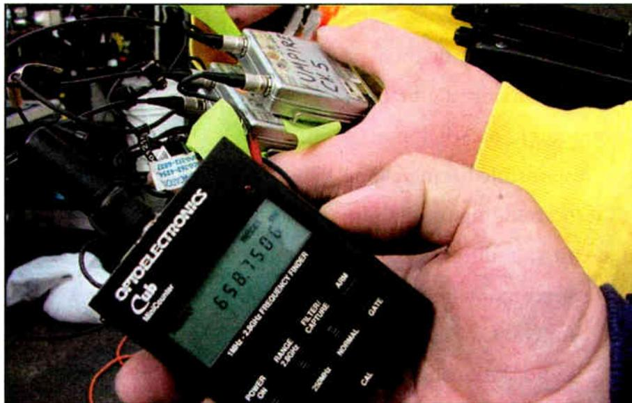
A GDC frequency counter verifies proper wireless mic operation on 658.7506. It pays to check; frequency-agile units could be tuned to the wrong channel accidentally.
