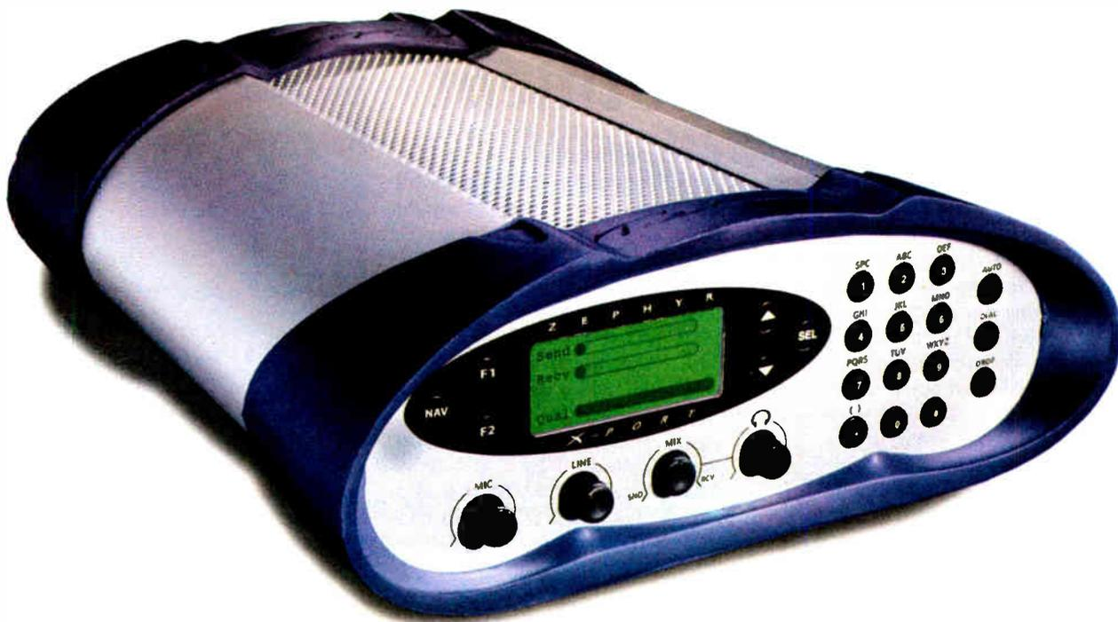
**More reliable** Xport doesn't rely on the off-the-shelf modems found in other POTS codecs. Instead, we developed a custom DSP modem optimized for live audio.
