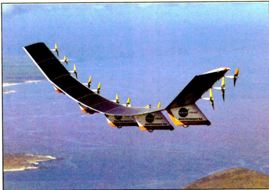
In flight, the flexible design of the Helios wing becomes apparent. The flying wing is shown in 2001 near the Hawaiian islands of Niihau and Lehua during its first test flight on solar power.
