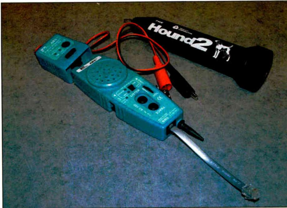
Fig. 3: Two types of signal/sensor units. The black Fox and Hound is a two-part signal generator/sniffer manufactured by Triplett. The sniffer is shown. Next to it is a Progressive Electronics device.
